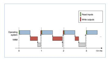
In each 1-ms cycle, the data are first read out of the object directory, which contains all settings and state values of the controller as the central database. Then the "operating system" is executed, such as the high-level functions of the motor controller and the field bus communication.
