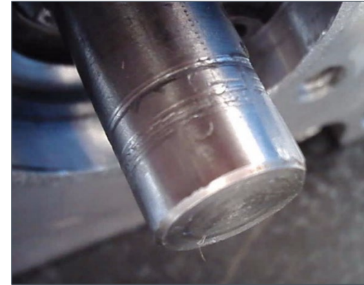
Failed motor shaft connection
