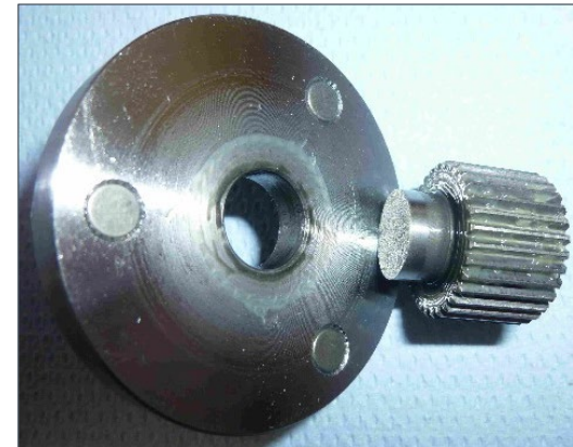
Failed press fit
