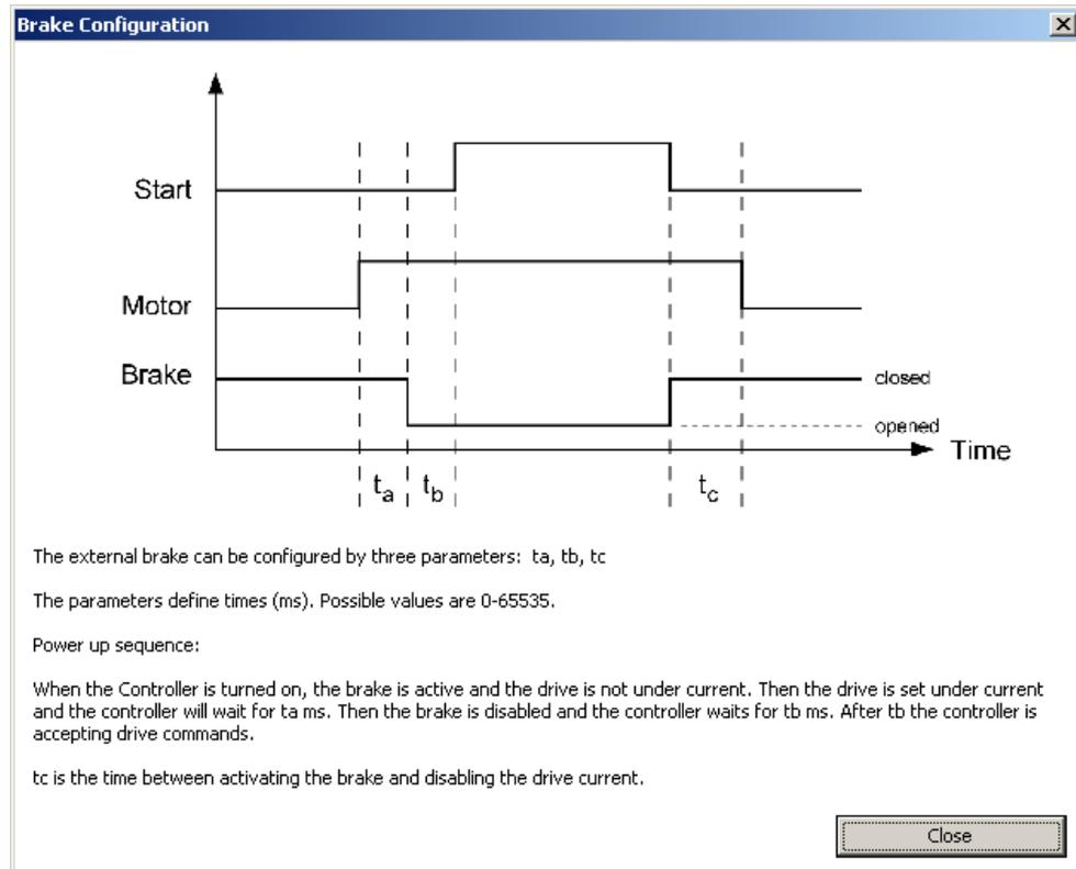
The external brake can be configured by means of the three  $t_a$ ,  $t_b$  and  $t_c$  parameters.
